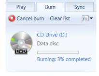
To burn the same files to a new disc, just insert a blank disc and click the burn button again.
